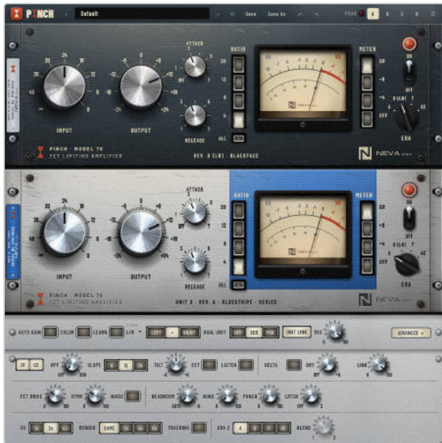
FIGURE 4 SER mode: unit 1 in Rev D (LN), unit 2 in Rev A. Strip and drawer take on unit 2's colours.
