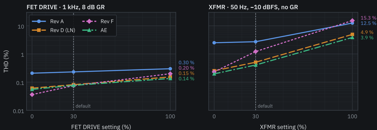
CHART H THD at FET DRIVE and XFMR settings of 0, 30 (default) and 100 %.
