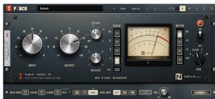
STEREO M/S with SIDE selected: the amber lamp marks the side being edited.
